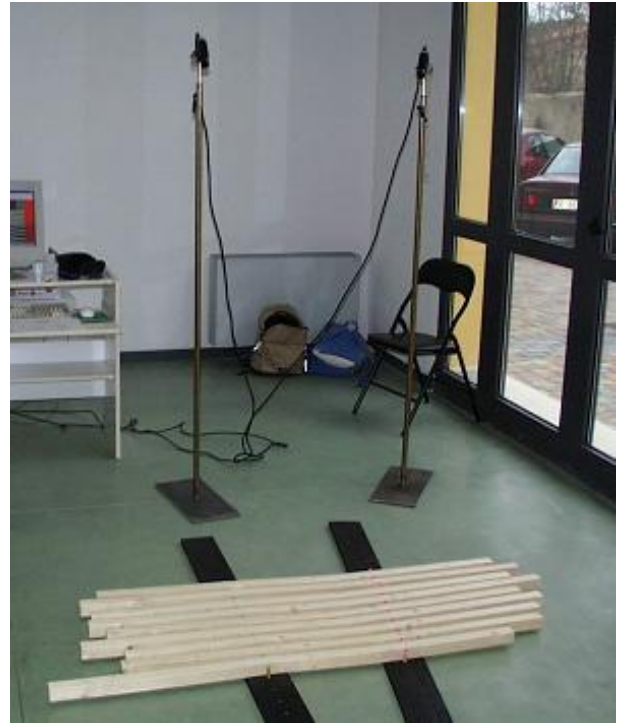
Figure 3: The system for pallet structuring that exploits colored markers.
