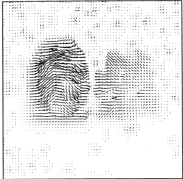
Fig. 12 Field resulting by applying the Horn and Schunck algorithm to the ROBOX sequence.
