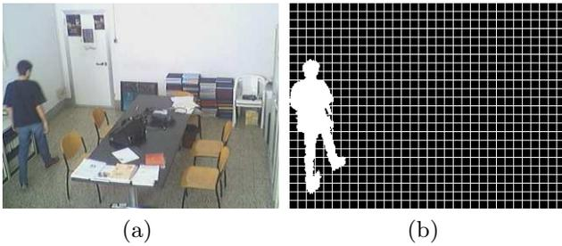
**Figure 1: An original frame (left) and the foreground frame with superimposed representation grid (right).**
