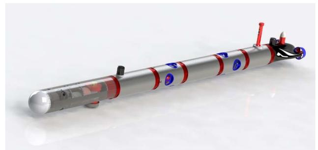
Fig. 1. Final CAD design of MARTA modular AUV
