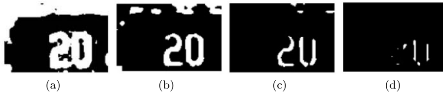
Fig. 7. Some results of our binarization method obtained by varying the threshold \tau . (a) \tau = 20 , (b) \tau = 50 , (c) \tau = 70 and (d) \tau = 90 . Best thresholding value \tau is 50.
